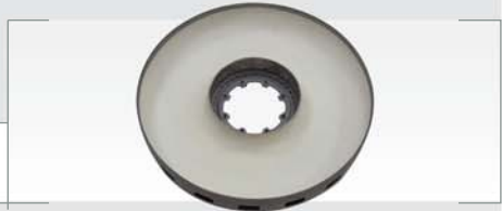
Helicopter Hub Sub-Assembly - Abradable Coating performed by Plasma technology using a Copper Aluminum Polyester.
