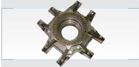
End Plate of a UAV Engine - A pure Molybdenum Coating performed by Arc-Spray for protection from Galling.
