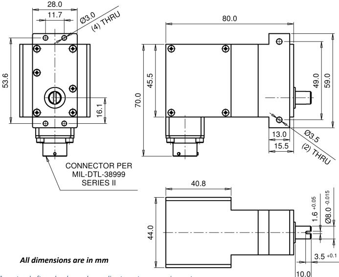
The outer shaft can be changed according to customer requirements.
