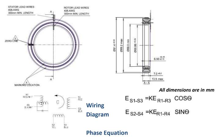
Where K – transformation ratio,  $\theta$  measured angle, deg.
